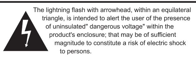
The lightning flash with arrowhead, within an equilateral triangle, is intended to alert the user of the presence of "uninsulated" dangerous voltage" within the product's enclosure; that may be of sufficient magnitude to constitute a risk of electric shock to persons.
